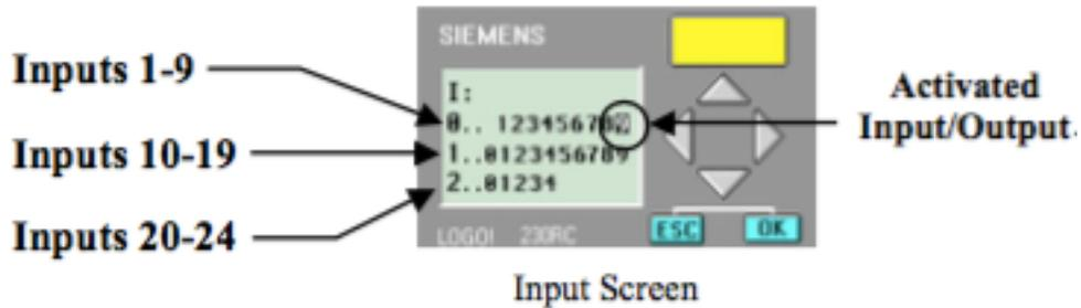
When lifting the floats check this screen to determine if the floats are wired into the correct position. When the floats are lifted a corresponding digit will be back lit. The input values are as follows:
